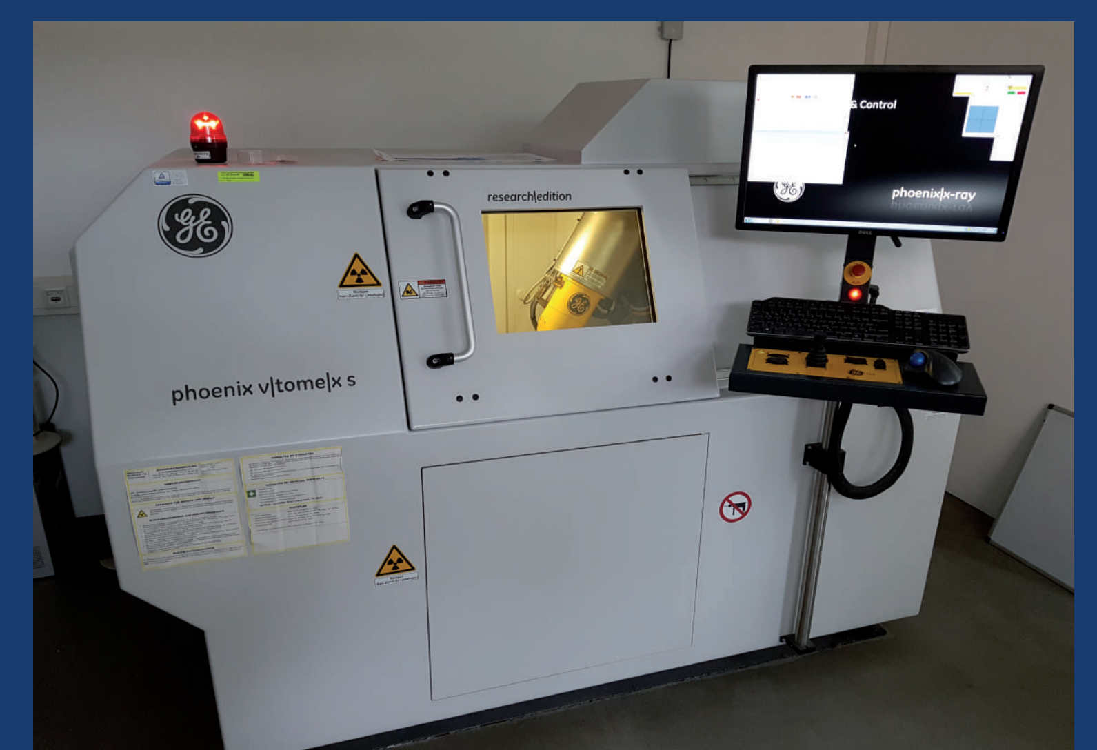
Fig.2. Prepared samples were scanned with the institute own micro-computed tomography. With this method samples are not destroyed and can be used for subsequent analyses.
